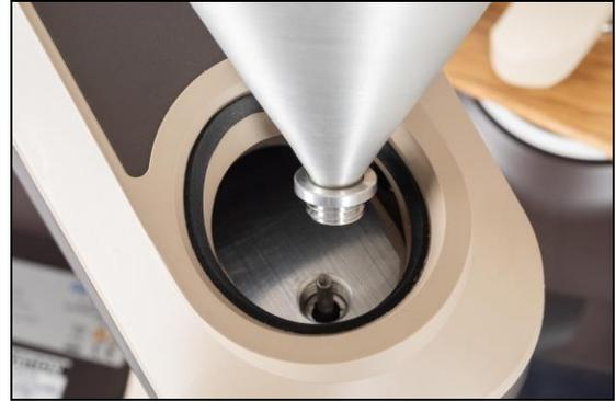
3. Insert the M3 Torx screw into the agitator hub; and then place the grit agitator on the agitator shaft inside the hopper. Secure by tightening the M3 Torx screw with the T-10 Torx Screwdriver.
