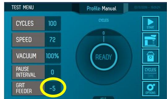
8. Repeat steps 4 – 6 a minimum of three times, and record values. The feed rate is calibrated when all three readings are 35 ± 5 grams.
