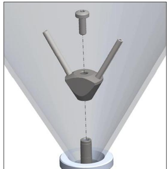
4. Lift the Taber vacuum pick-up nozzle into its upright rest position. Insert the offset, front orifice vacuum nozzle into the vacuum port opening.
