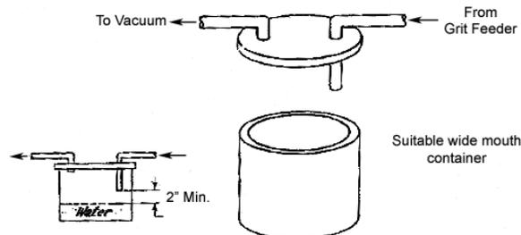
A tight seal is not required between the container and the lid. Also, the inlet pipe to the water trap should be far enough away from the water surface
